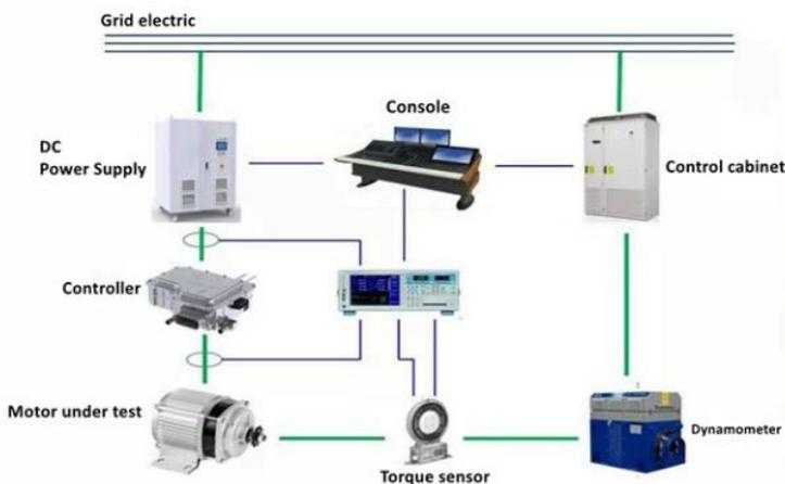
It satisfies the test of different stages of drive motor system development, model test, reliability test and factory inspection.
