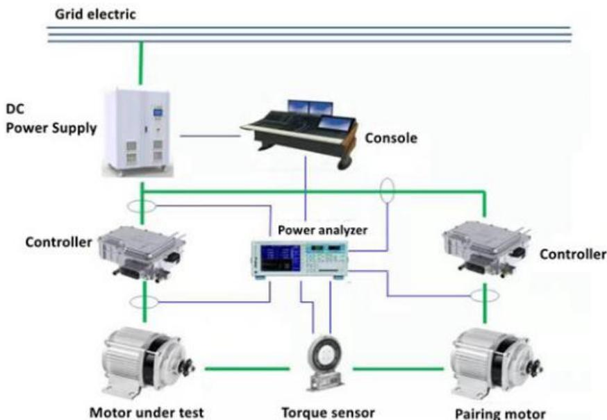
It is suitable for the test of the same type of motors, which realizes the recycling of energy.
