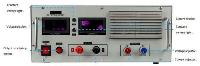
Main power switch. Positive output terminal. Negative output terminal.
